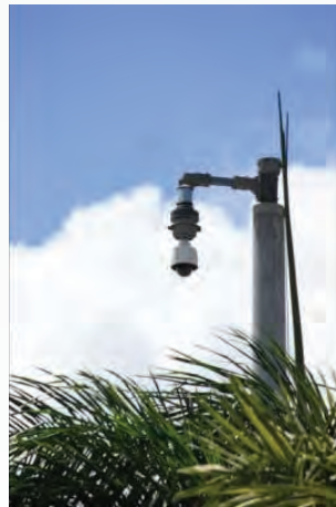
Figure 6-8: Wireless bluetooth reader
